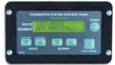
DRIVER CONTROL PANEL
